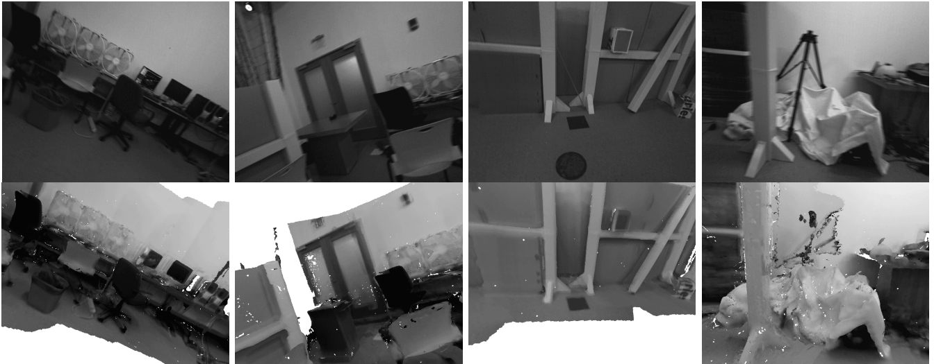
Fig. 7: The Aggressive 1 sequence, where the first row shows the camera images and the second row shows rendered images at the estimated poses. Despite the imperfections in the mesh, shown as white holes in the rendered views, renderings at our pose estimates accurately match the camera images, indicating successful camera tracking. Refer to https://groups.csail.mit.edu/rrg/star for the full sequence.
